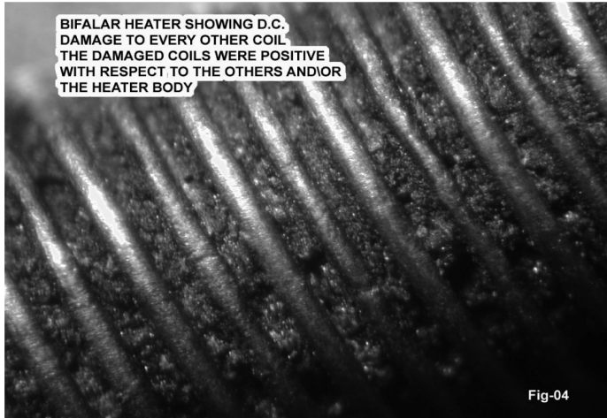
Figure 4 shows the D.C. damage to the bifilar shown in Figure 3. This heater is grounded to the heater can. However, heater power lead polarity makes no difference as each turn is the opposite polarity to its neighbor.
